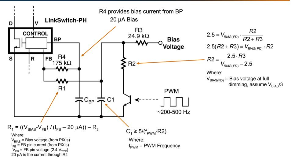
Dimming range can be increased by simultaneously decreasing FB Pin current and increasing V Pin current
