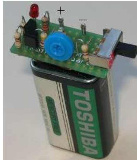
The regulator connected to a 9v battery
