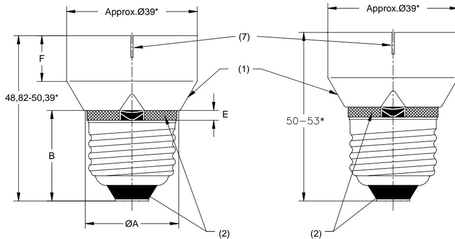
The E26/50x39 version is used in North America while the E26/51x39 version is used in Japan.
