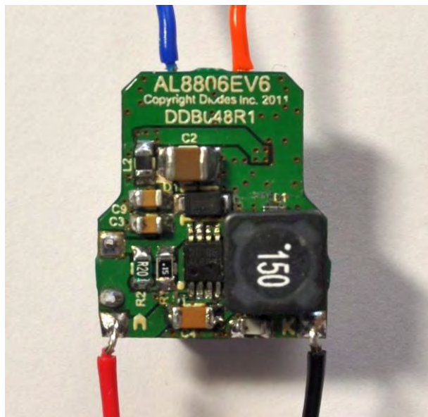
Figure 8. AL8806EV6 evaluation board (Top)
