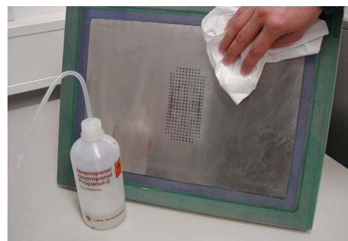
Fig. 3: Cleaning of the screen print template
