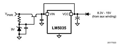
FIGURE 7. Start-Up Regulator for V<sub>PWR</sub> >100V
