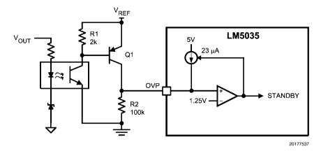
FIGURE 14. Latched Load Over-Voltage Protection
