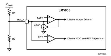
FIGURE 10. Basic UVLO Configuration
