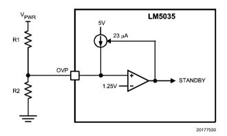
FIGURE 11. Basic Over-Voltage Protection
