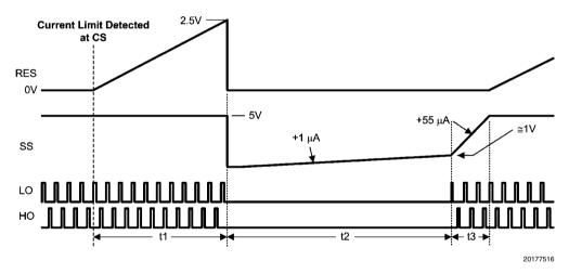
**FIGURE 3. Current Limit Restart Timing**
