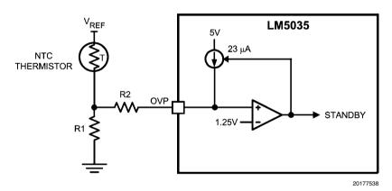
**FIGURE 15. Remote Thermal Protection**
