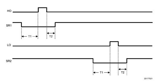
FIGURE 5. HO, LO, SR1 and SR2 Timing Diagram
