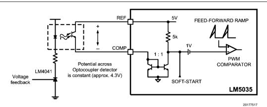
FIGURE 4. Optocoupler to COMP Interface
