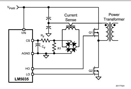
FIGURE 8. Current Sense Using Current Sense Transformer
