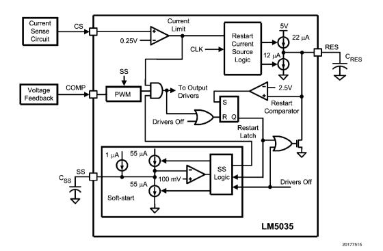
**FIGURE 2. Current Limit Restart Circuit**
