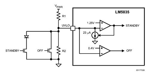
FIGURE 13. Remote Standby and Disable Control
