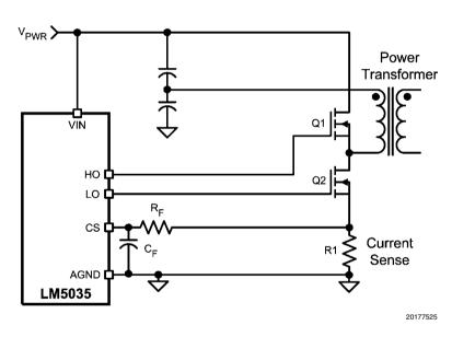
FIGURE 9. Current Sense Using Current Sense Resistor (R1)
