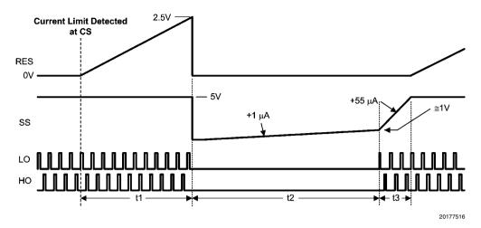
FIGURE 16. Hiccup Over-Load Restart Timing
