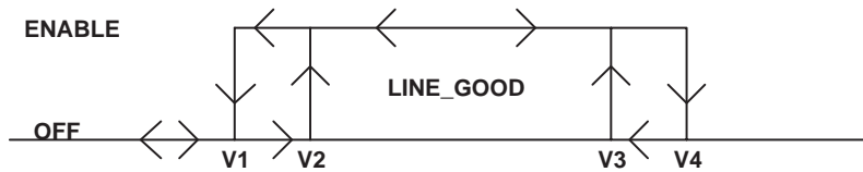
Figure 2. Line UVLO and OVLO Operation
