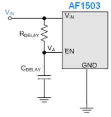
For example, setting V<sub>IN</sub>=24V, R<sub>DELAY</sub>=100KΩ, C<sub>DELAY</sub> =0.1uF. The start-up delay time can be calculated as below:
