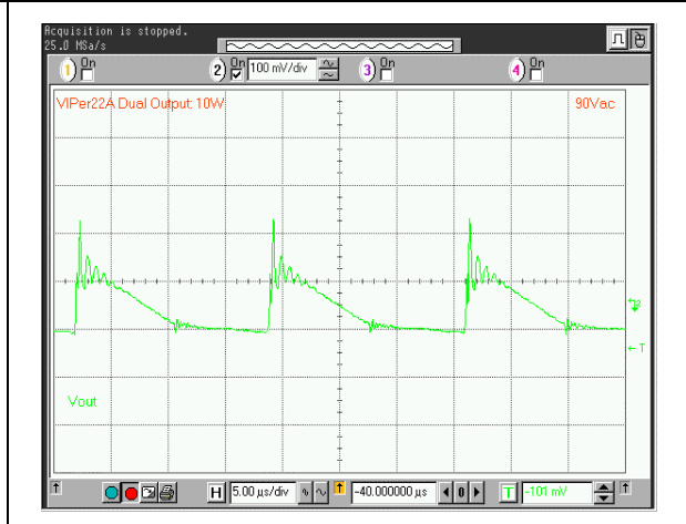
Figure 12. Switching ripple for 12V output
