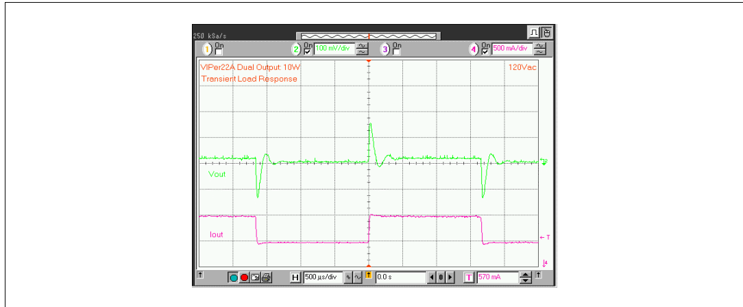
Figure 13. Transient load response
