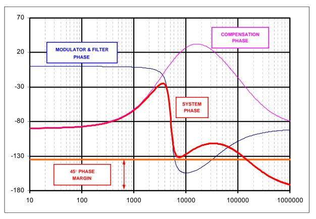
FIGURE 13. BODE PLOT OF THE TYPE III SYSTEM EXAMPLE
