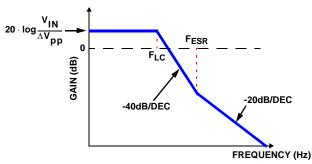
FIGURE 5. OPEN LOOP SYSTEM GAIN
