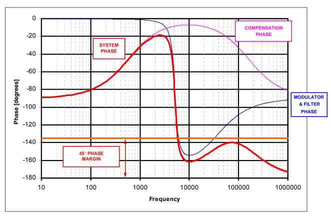
FIGURE 12. BODE PLOT OF THE TYPE II SYSTEM EXAMPLE
