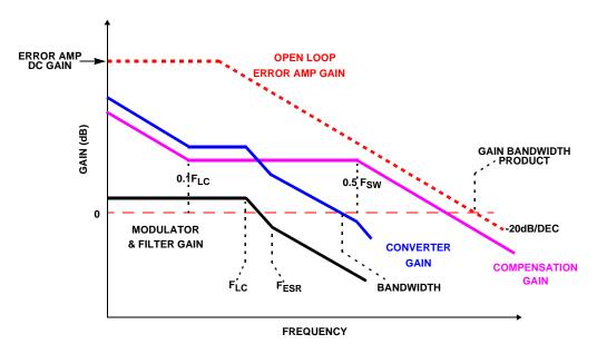
$$GAIN_{dB}(f) = GAIN_{MODULATOR} + GAIN_{FILTER} + GAIN_{TYPEII}$$
