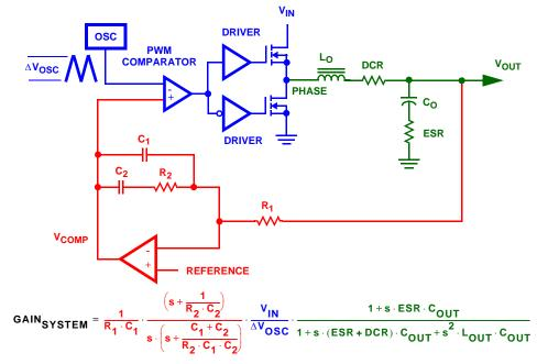
FIGURE 7. CLOSED LOOP SYSTEM WITH TYPE II NETWORK
