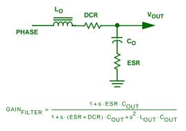
FIGURE 3. THE OUTPUT FILTER
