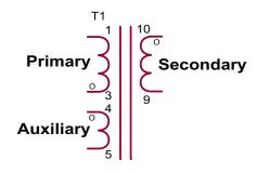
$L_{PRIMARY} = 1.1mH \pm 8\%$ Leakage inductance = 8% of  $L_{PRIMARY}$
