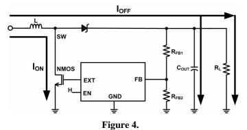
For the PWM control method, the switching frequency  $(f_{sw})$  is fixed and the  $V_{OUT}$  voltage is held constant according to the ratio of the ON time and OFF time (ON duty) of NMOS in each period.
