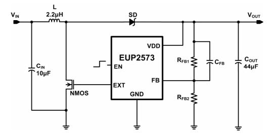
Figure 2. Connecting VDD to  $V_{\mbox{\scriptsize OUT}}$
