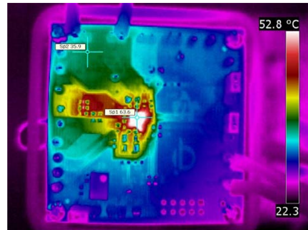
Case Temp = 63.6°C with 5V OUT
