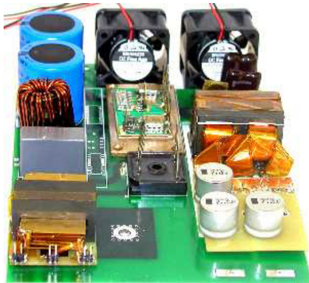
Figure 5-31. IPEM-based front-end converter with 400 kHz PFC and 400 kHz LLC.
