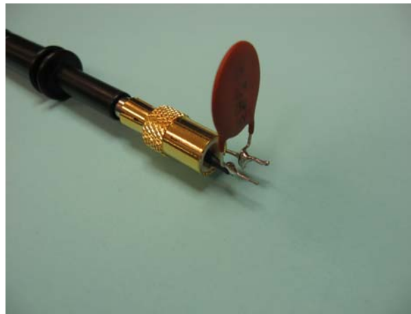
Figure 55 – Oscilloscope Probe with Probe Master ( www.probemaster.com ) 4987A BNC Adapter. Modified with wires for ripple measurement, and one parallel decoupling capacitor added.)
