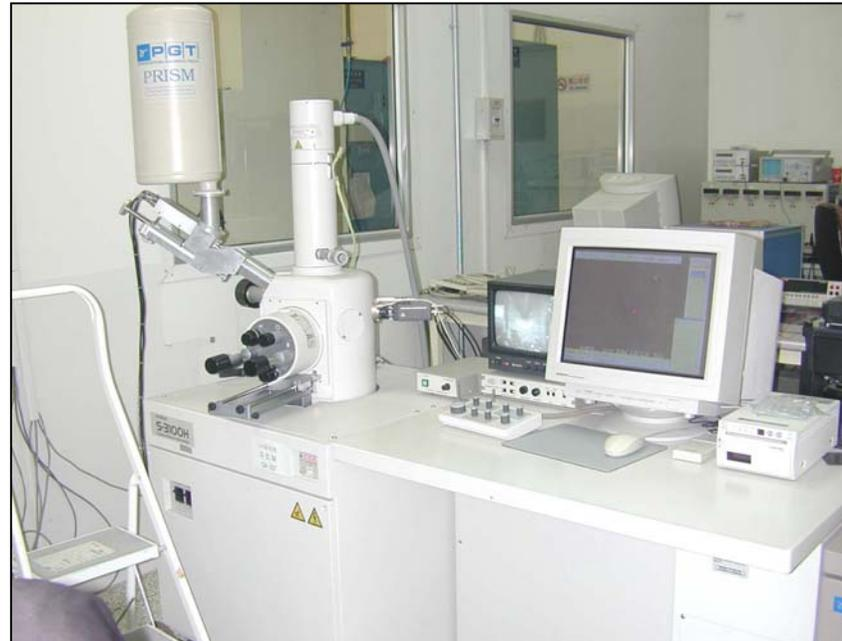
**SEM imaging system, up to x10K magnification**
