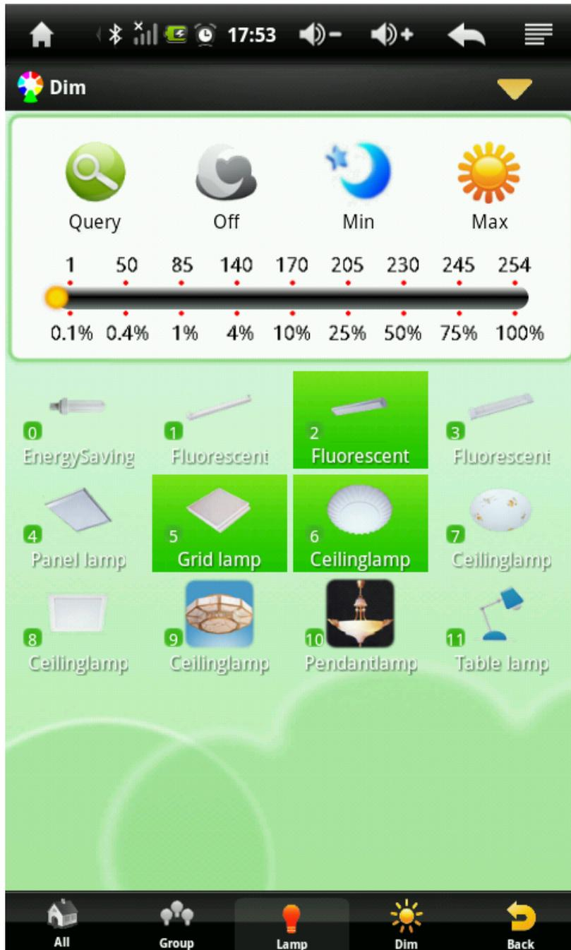
UI Dim: you can select ALL lamp, groups or lamps, and do the action of direct ARC, indirect dim or goto a scene.
