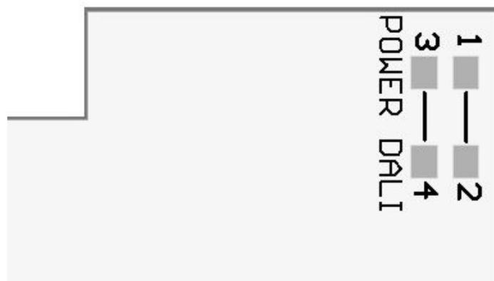
( connect between 1,2 and connect between 3,4 as above to power DALI line from DC15-16V source)
