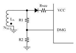
$$V_{O\_STR} = \frac{N_S}{N_A} \times 3 \times \frac{R_I + R_2}{R_2}$$
