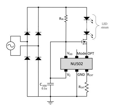
DC PWM dimming application (No leakage current)
