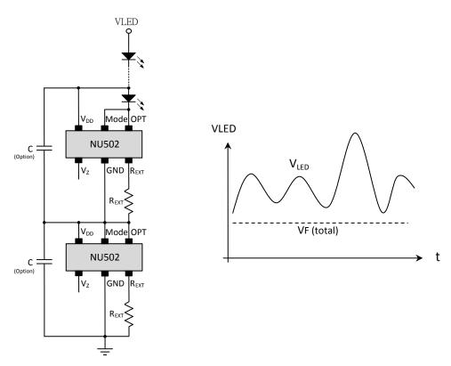
By cascade mode, two or more NU502 in series can absorb higher voltage variation in lighting system. Each NU502 can share about 12 volts redundant. The total voltage variation range that system can work is calculated by following equation.
