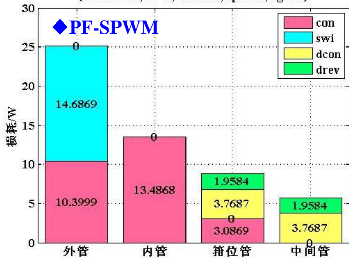
3L-ASNPC器件损耗分布图 (PF-SPWM, PF=1, P o =5kW, U pvmin , U gmin )
