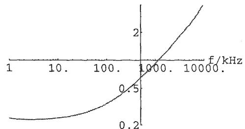
Fig. 5: Input resistance of power transformer, secondary side shorted
