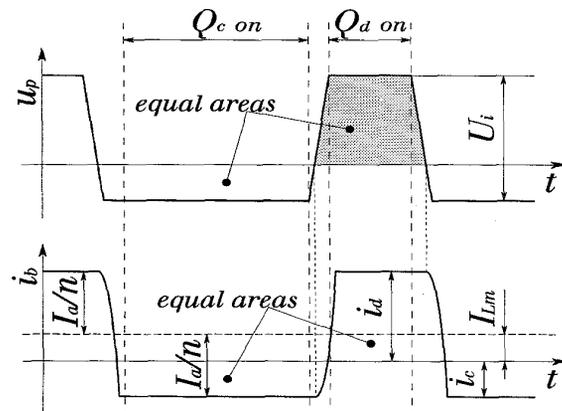
Fig. 2: Typical waveforms for the ASHB at soft switching (mode I)
