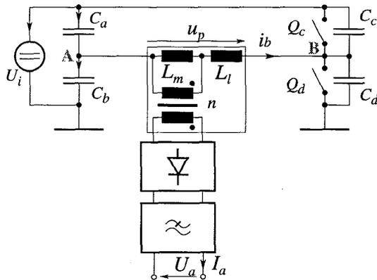
Fig. 1: Typical halfbridge topology whereby the shaded box represents the transformer with leakage and magnetizing inductance.
