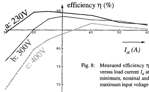
Fig. 8: Measured efficiency  $\eta$  versus load current  $I_a$  at minimum, nominal and maximum input voltage
