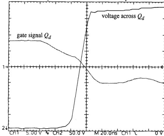
Fig. 6: Measured waveforms of ASHB at nominal power (mode I) operation conditions: 380V/5V – 60A, 500kHz
