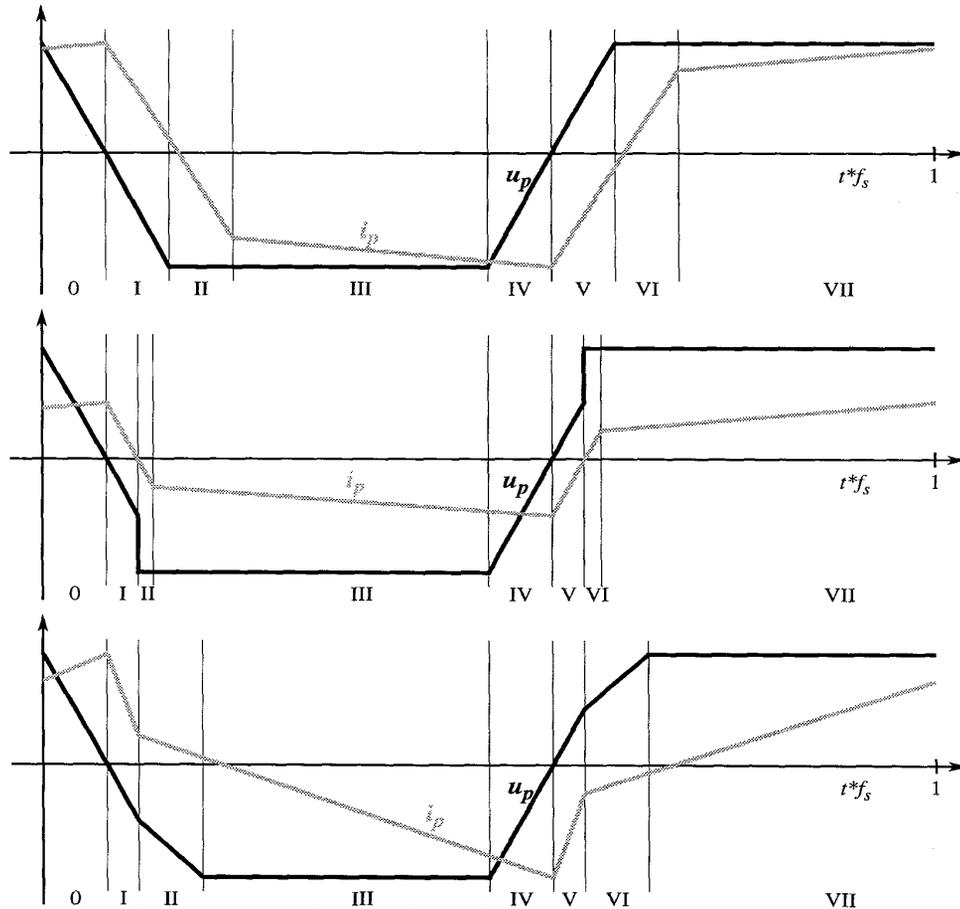
Fig. 4: Principal waveforms of primary current  $i_p$  and inverter voltage  $u_p$  for a) mode I, b) mode II, c) mode III and relation between intervals and states: 0=Z2a, I=Z3a, II=Z11, III=Z9, IV=Z1b, V=Z3b, VI=Z7, VII=Z6
