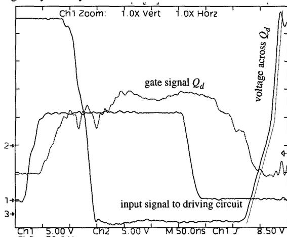
Fig. 7: Measured waveforms of ASHB at low power (mode II) operation conditions: 350V/5V – 6A, 500kHz
