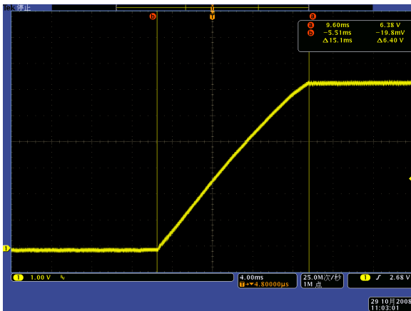
Figure 13. Rise time, 115Vac, Full Load, 1V, 4ms/div
