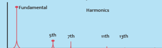
Typical Harmonic Distortion of PWM Inverter With 5% Impedance Reactor
